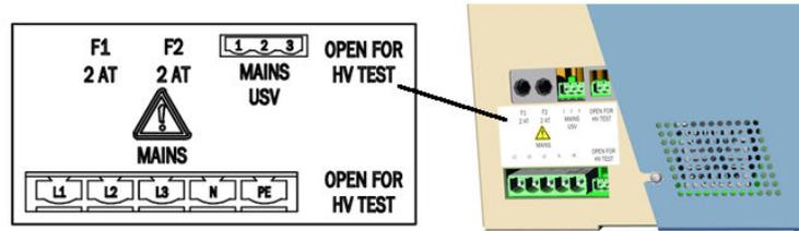
Figure 19: Power supply connections
