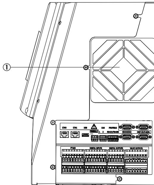
Figure 18: Electronic housing (right side)
