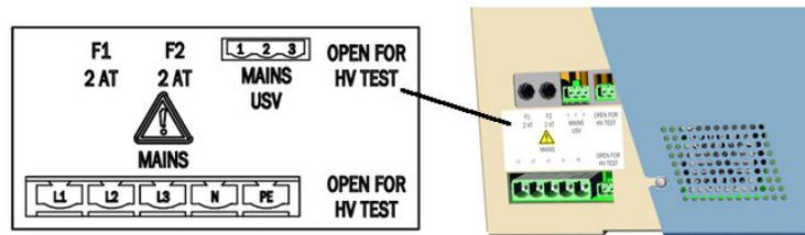
Figure 12: Power supply connections
