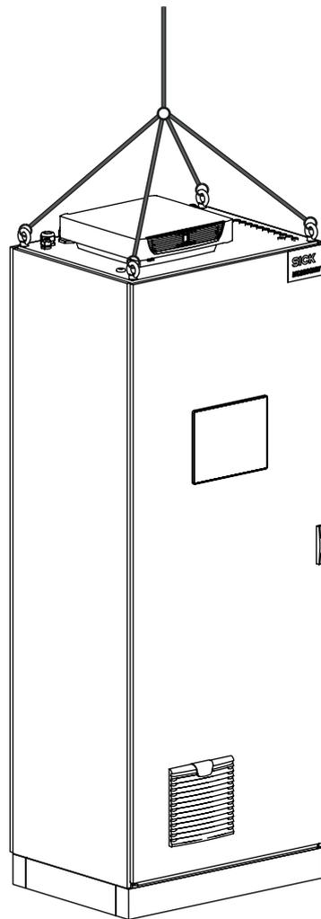
Figure 6: Analyzer cabinet suspension
