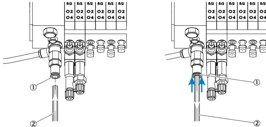
Figure 9: Push-in fitting with retaining ring
