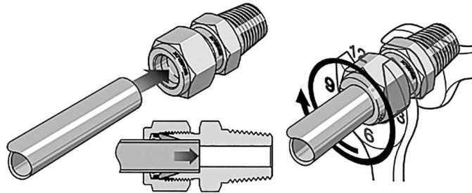
Figure 8: Clamping ring screw connection
