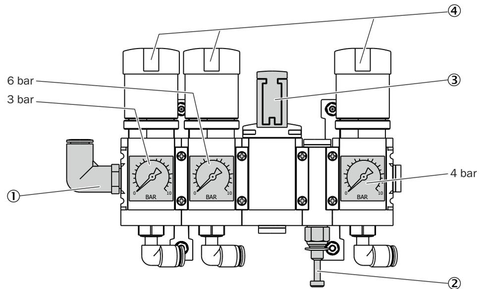
Figure 10: Pressure reducer module
