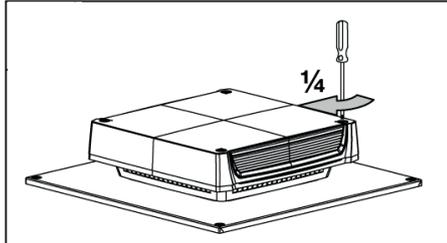
**Replacing the lower filter pad:**
