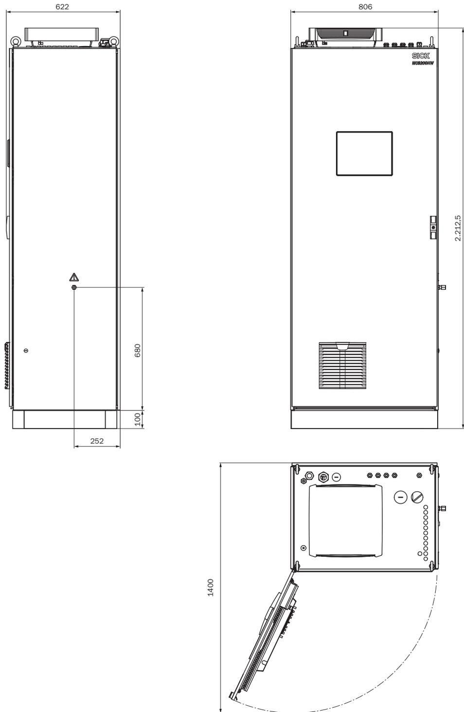
All dimensions in the dimension drawing are in mm.
